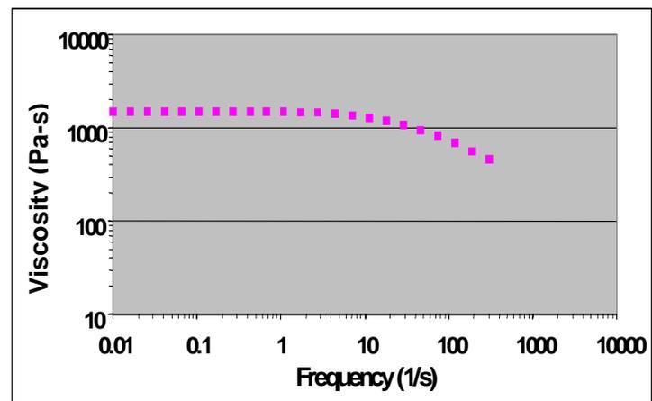
Figure 5. Melt viscosity of a 24 MFR Vistamaxx™ specialty elastomer at 190 °C
