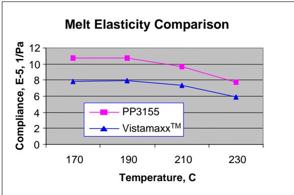
Figure 6, Compliance of Vistamaxx™ vs. PP homopolymer
