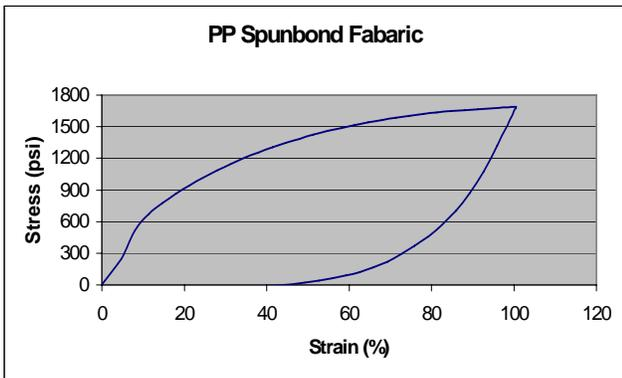
Figure 7. Hysteresis curve for PP homopolymer spunbond fabric
