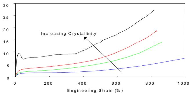
Figure 2. Stress-strain curve of specialty elastomer product family
