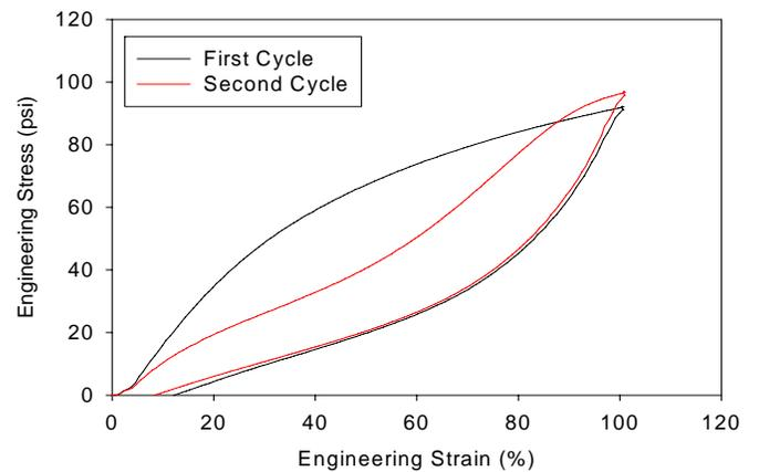
Figure 11. Stress-strain plots of a melt-blown fabric made from Specialty Elastomers
