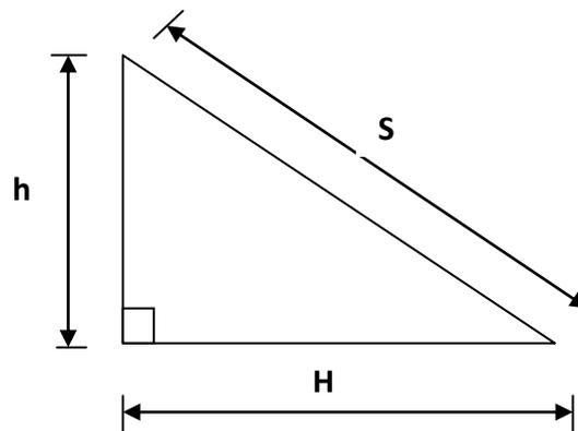
Fig. (3.3): Measuring the horizontal distance using the inclined distance and the head diff.
