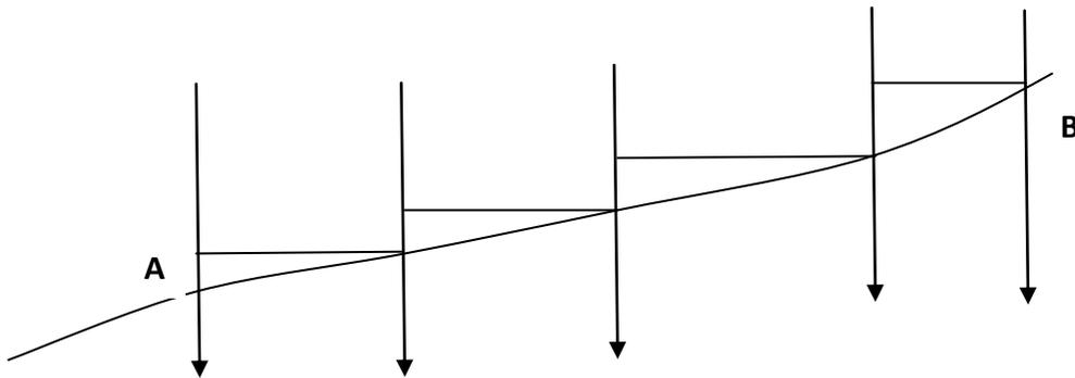
*Fig. (3.1): Measuring the distance in case of inclined land*
