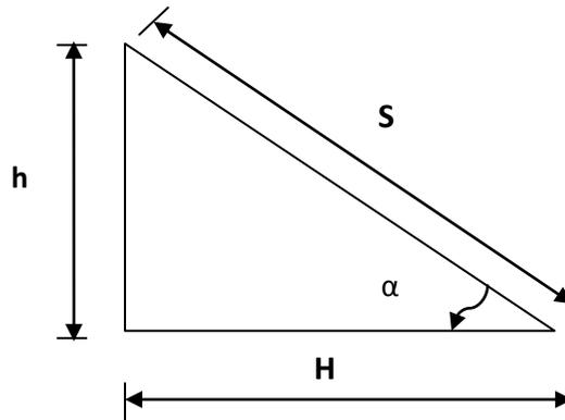
Fig. (3.4): Measuring the horizontal distance using the vertical angle and the head diff.
