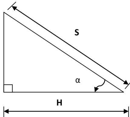
Fig. (3.2): Measuring the horizontal distance using the inclined distance and vertical angle
